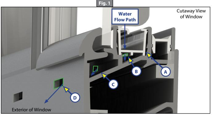
A leak is present if there is visible water on an interior glass surface of a fixed component of the window, or if water enters the interior of the unit through the window.
